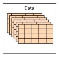
In the picture above, the data is stored as a three dimensional dataset of size 4 x 5 x 6 with an integer datatype. It contains attributes, *Time* and *Pressure*, and the dataset is chunked and compressed.
