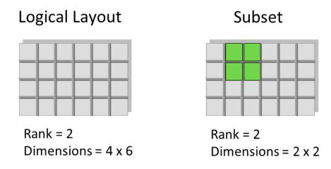
The dataspace is used to describe both the logical layout of a dataset and a subset of a dataset.
