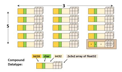
This is an example of a dataset with a compound datatype. Each element in the dataset consists of a 16-bit integer, a character, a 32-bit integer, and a 2x3x2 array of 32-bit floats (the datatype). It is a 2-dimensional 5 x 3 array (the dataspace). The datatype should not be confused with the dataspace.
